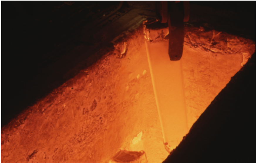
Figure 10, ASCOMETAL has employed flameless oxyfuel to reduce the number of soaking pit furnaces from 13 to 9 for the same production volume. This is paired with fuel savings, more uniform heating of the ingots and less emissions of CO 2 and NO x .
