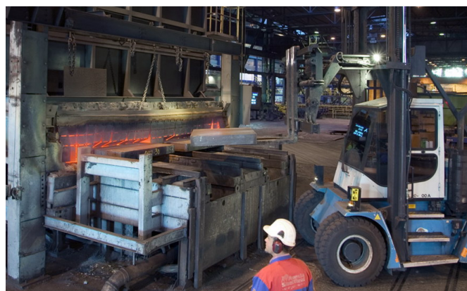
Figure 2, Outokumpu Stainless in Sweden increased their heating capacity in the existing walking beam furnace by 40-50% when implementing flameless oxyfuel. With this investment in an existing furnace the plate mill could accumulate production volumes from another site.
