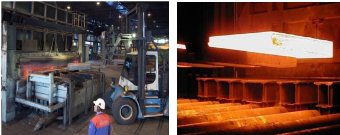
Figure 4. Outokumpu in Sweden increased its heating capacity in the existing walking beam furnace by 40-50% when implementing flameless oxyfuel. With this investment in an existing furnace plate mill could accommodate production volumes from another site.
