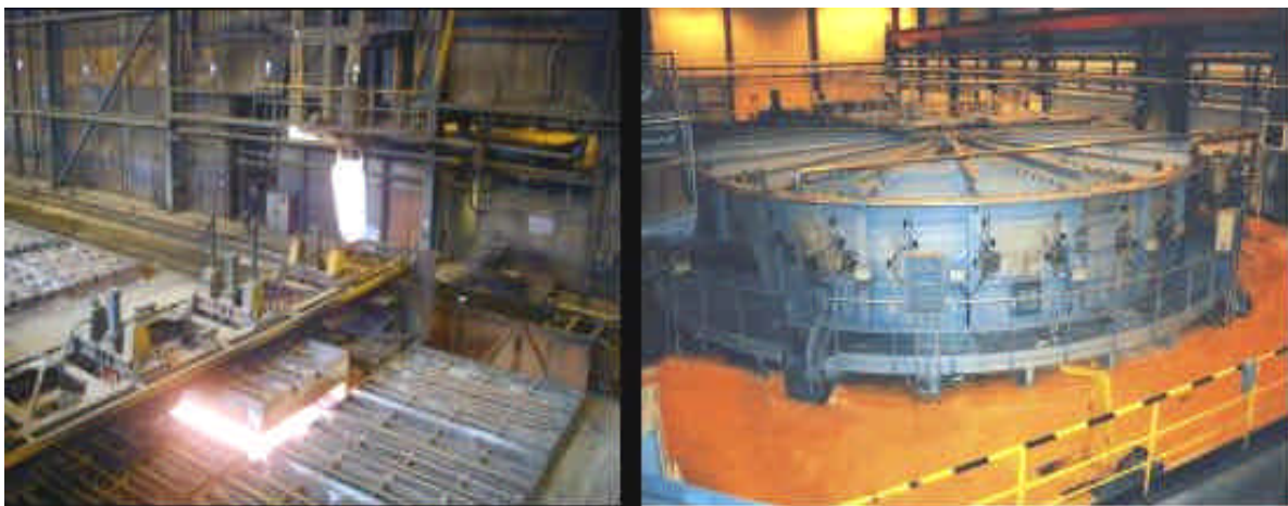
Figure 2: Ovako, Hofors works, Sweden, uses oxyfuel in 40 pit and 2 rotary-hearth furnaces for greater throughput capacity, providing flexibility and better-planned maintenance activities.
