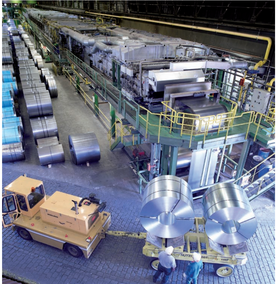
DFI oxyfuel for implementation in existing galvanizing line, at ThyssenKrupp Steel, Finntrop, Germany, 2006.
