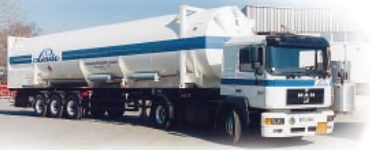
Tanker delivering liquid hydrogen
