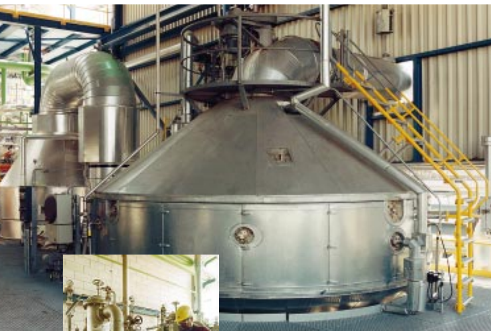
Oxidation of ammonia for production of nitrogen monoxide
